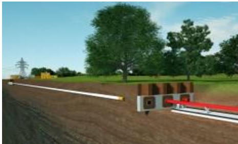
AVNS 350 XB being operated in conjunction with the E-Power Pipe method
