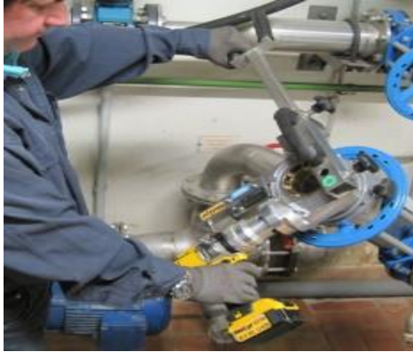
Accutiger slide-gate valve power wrench
