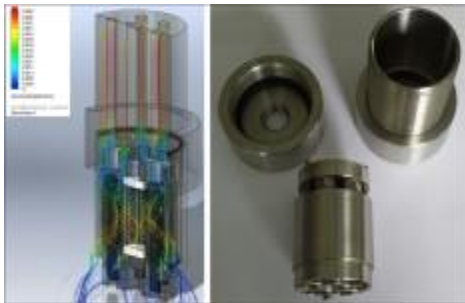
Fluid-flow simulation (on the left) and mounting of collectors in the RPS
